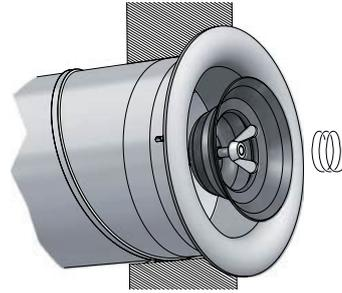
2- Use of an anemometer with cone to detect air flow: Place the cone over the valve and detect the air flow on the display. Rotate the front plate to adjust the air flow. Place the anemometer over the valve again and detect the air flow on the display. Repeat if necessary.
